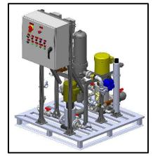
Capture and use or reuse your shower and rain water with our fully automatic treatment systems. Systems come fully inclusive with process pump, backwash pump, prefiltration, secondary polishing and disinfection. Standard design up to 30,000 gallons per day with full PLC control and remote login capabilities; custom manual and automatic designs available by request
